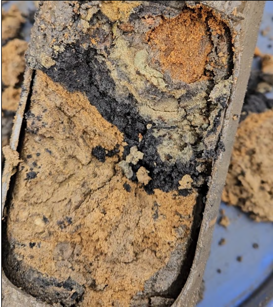
IMAGE NO. 3: Example of sand fill encountered at hand auger borings
